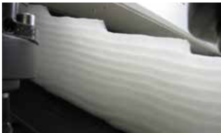
The crosslapper's CROSSMASTER system eliminates higher web weights in the edge area
