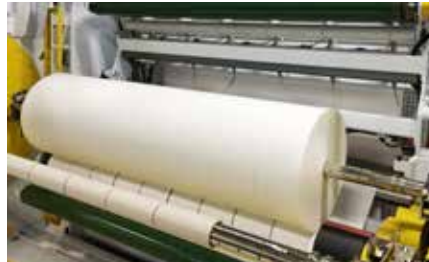
Precisely adjusted tension allows for winding sensitive materials such as cotton pads
