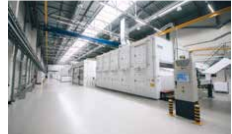
Highest evaporation capacity: a 5-drum dryer in a heavy duty cotton nonwoven line
