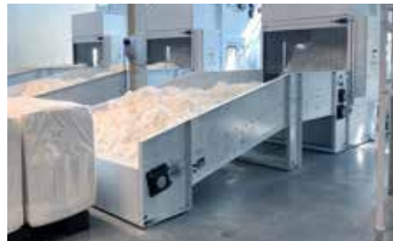
Bale opener TBL-BO is adjustable to a broad range of fibers
