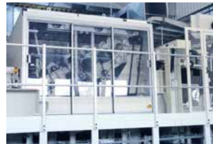
NCA airley card for webs with a balanced MD/CD ratio
