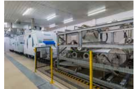
A small-sized AquaJet entangles the homogeneous web delivered by several TC cards.
