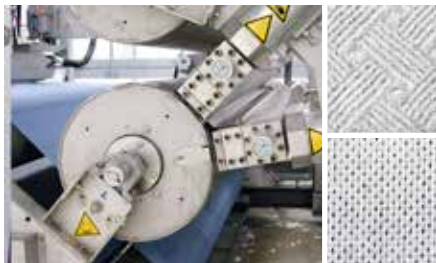
A finely tuned system: AquaJet spunlace drum and jet heads
