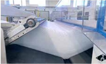
Forming the perfect web by automatic web weight regulation
