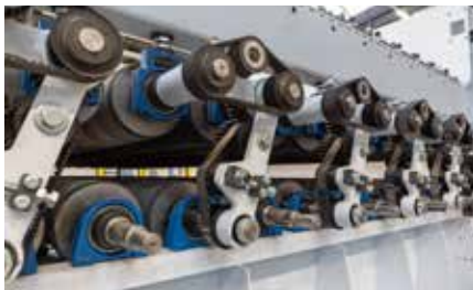
Giving a crosslapped web the final touch: TWF-WD web drafter
