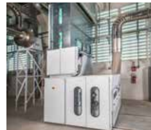
The fine opener TBL-FO for natural fiber processing in natural or recycled fiber lines
